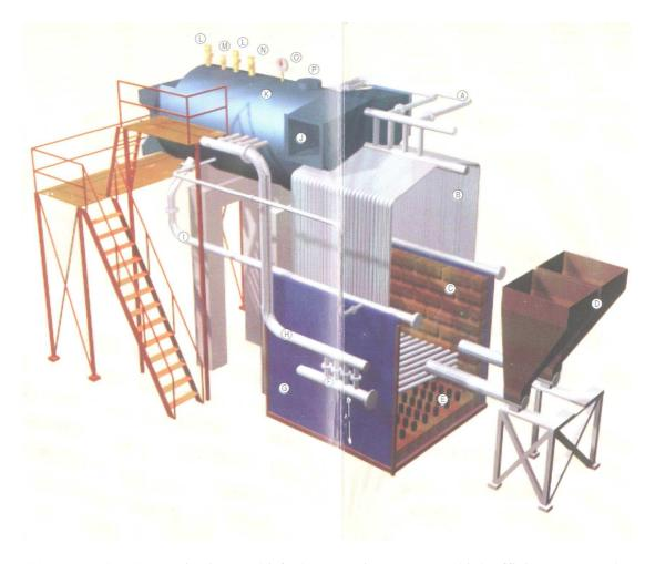
COMBIPAC – CPF series is a multi-fuel composite, two pass, high efficiency, natural circulation, balance draft, packaged boiler working on FIXED GRATE TECHNOLOGY and other ADVANCE COMBUSTION SYSTEM.
